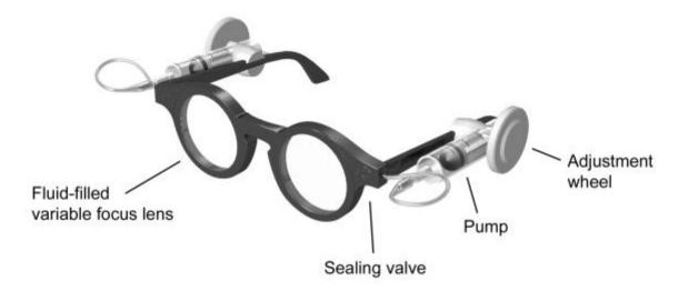
The refractive index of silicone oil is 1.406. To adjust the lens, you turn a knob that pumps fluid into or out of the chamber.
